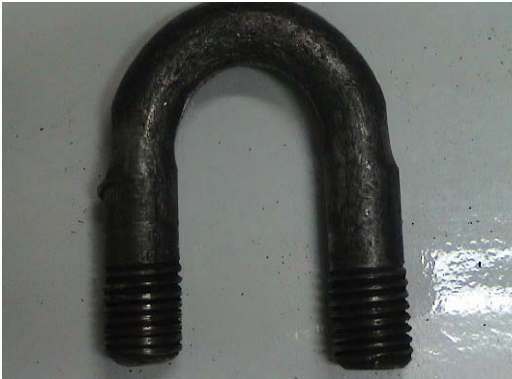
Figure 3 – Threads are damaged due to either incorrect retaining nuts or “picking up” while the nuts were fitted. DO NOT USE.
